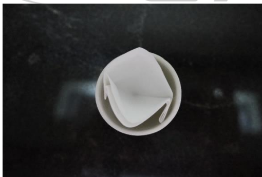
c) Place inside crucible with point pushed against bottom
