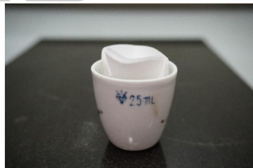
c) Place inside crucible with point pushed against bottom
